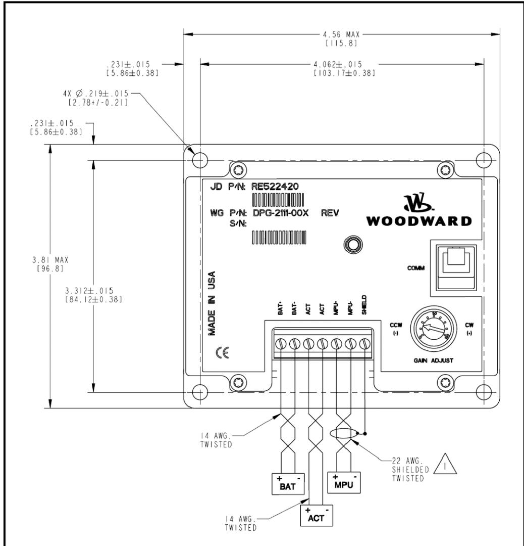
Figure 1. Wiring Diagram for DPG-2111- 001 Controller
