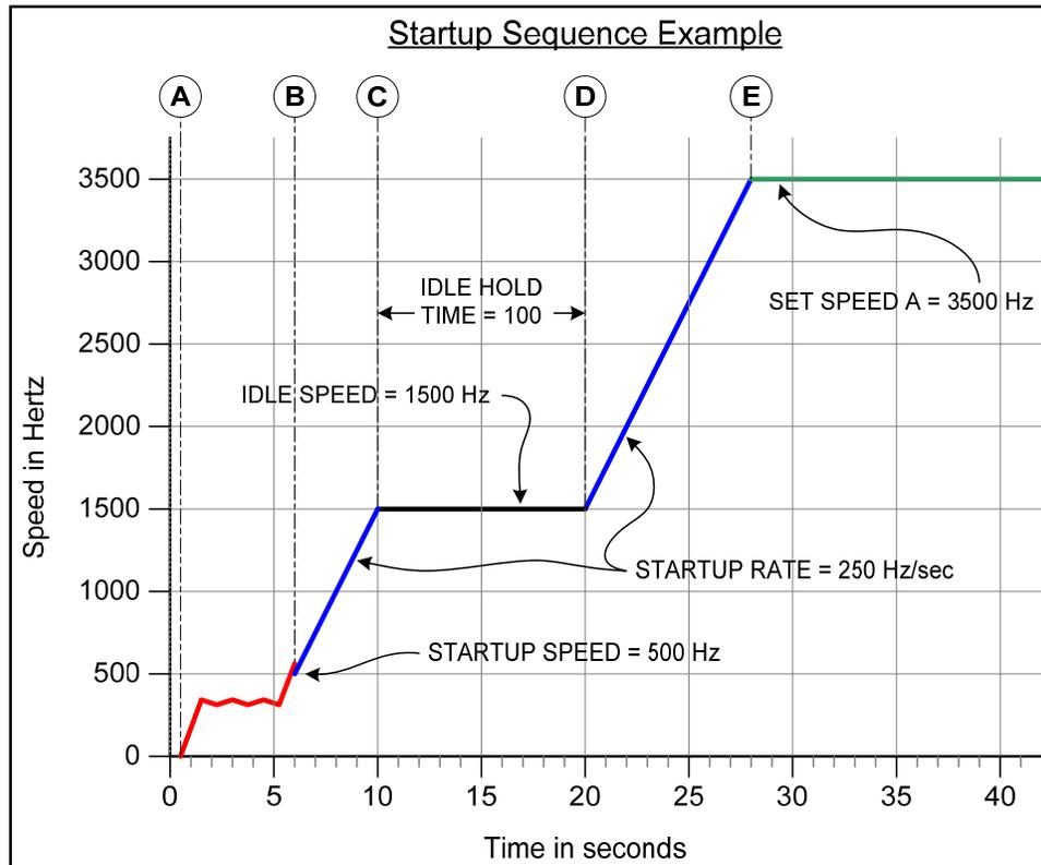
Engine cranking begins at point A. After a short time, the engine starts and at point B the engine speed exceeds the STARTUP SPEED (the initial target speed) and the controller now considers the engine to be running.
