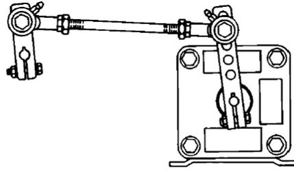
Figure 2-4. Linear Linkage
