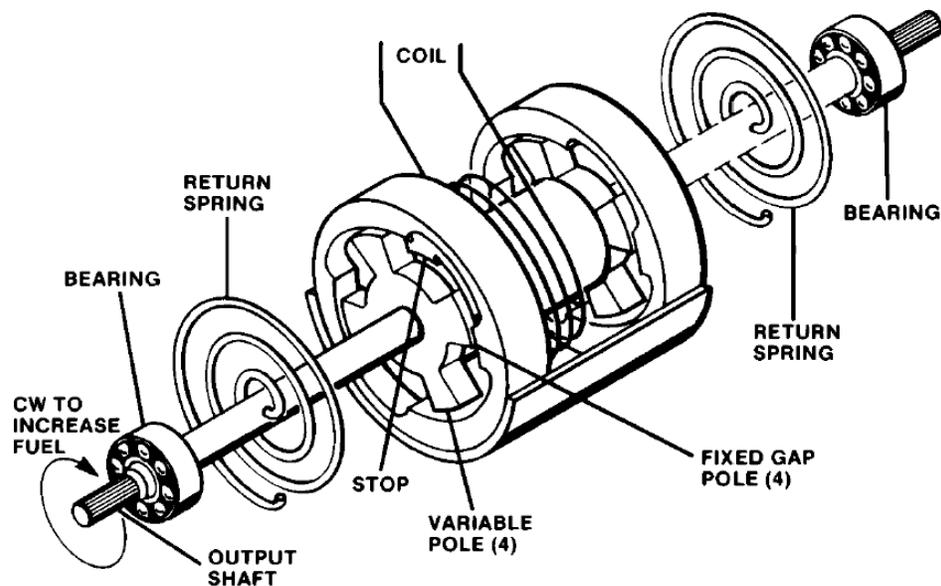
Figure 4-2. Actuator Schematic
