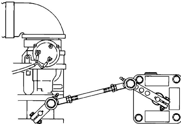
Figure 2-6. Carburetor Compensating Linkage at Maximum Fuel
