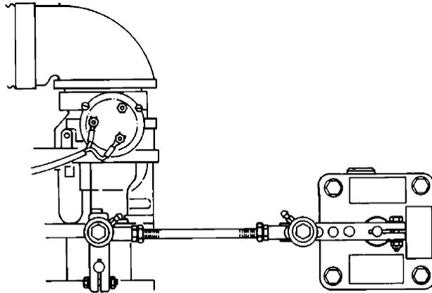
Figure 2-5. Carburetor Compensating Linkage at Minimum Fuel
